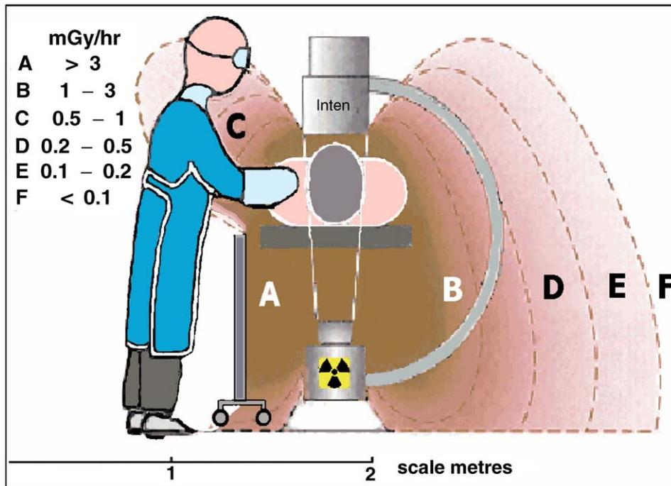
Figure 5 With the receptor close to the patient and with a mobile or table suspended shield the scatter is significantly reduced towards the surgeon. Compare with Figs. 3 and 4.
