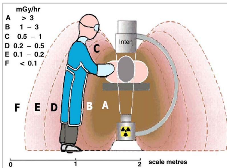
**Figure 4** With the X-ray generator beneath the operating table the receptor can be placed closer to the patient so reducing the primary radiation exposure to the patient. The scatter towards the surgeon's head and neck is significantly reduced. Compare with Fig. 3.
