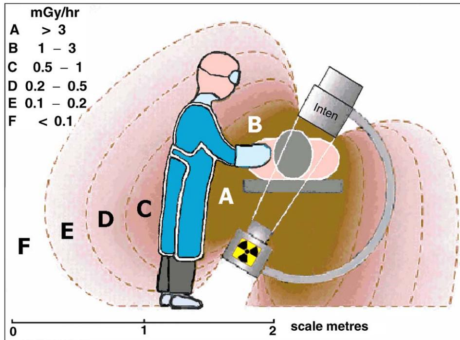
**Figure 7** With the C arm angled 15 degrees with the image receptor away from the surgeon the scatter to the surgeon's head and neck increases. The position of the generator interferes with the use of a rigid table suspended or mobile screen. The scatter to an assistant on the opposite side decreases but the assistant must utilise full protection methods.
