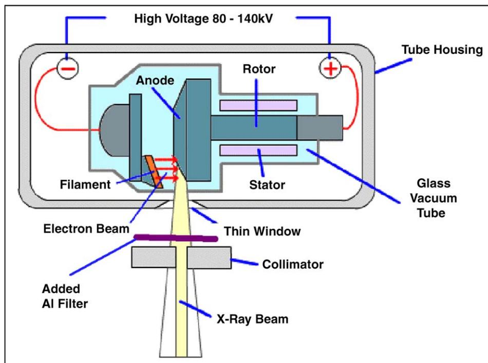
**Figure 1** Schematic diagram of an X-ray tube assembly, showing the various components including the important aluminium filter.
