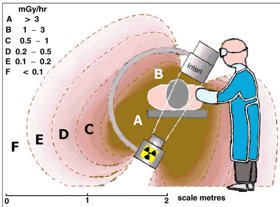
Figure 6 With the C arm angled 20 degrees with the image receptor towards the surgeon and adjacent to the patient the scatter to the surgeon's head and neck is reduced. A table suspended or mobile screen would reduce the scatter to minimal levels (see Fig. 5). The scatter to the assistant on the opposite side of the table is increased and the assistant must move away during exposures.
