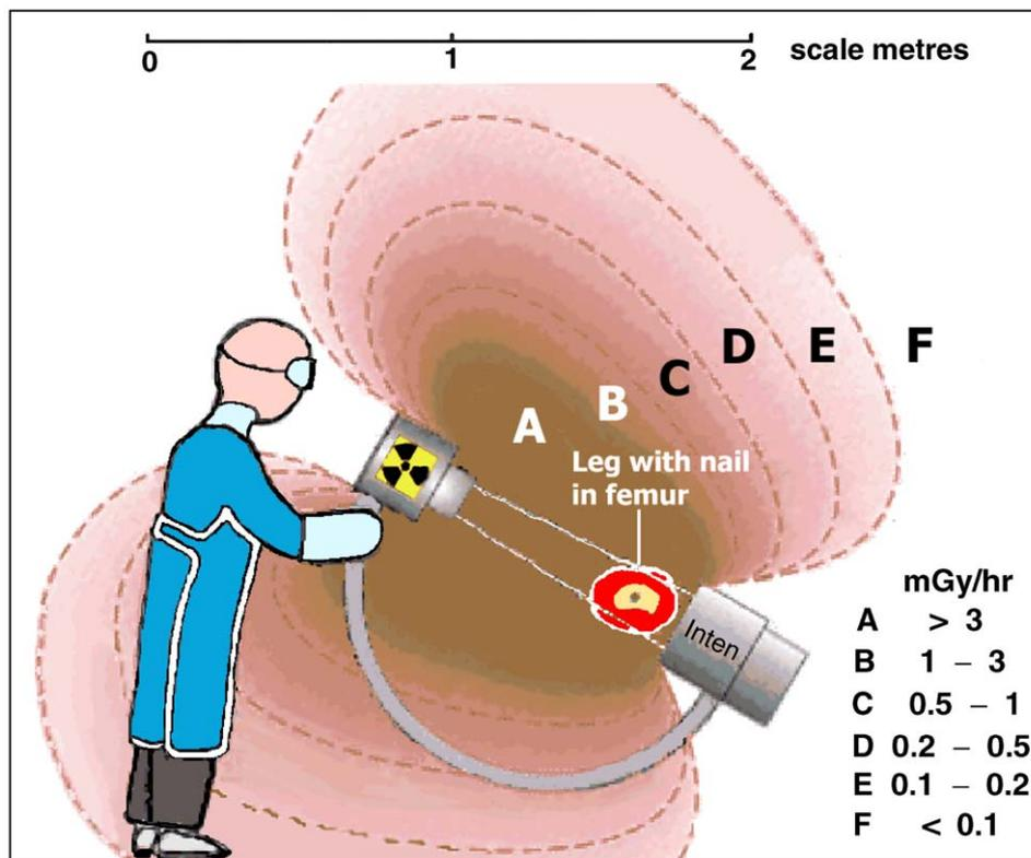
**Figure 8** The C arm is positioned to allow the surgeon operative access to the lower limb to insert cross screws to the lower femur or tibia. The closeness of the receptor to the limb and the small volume of tissue minimises radiation dose and back scatter. With real time operative manoeuvring the surgeon must avoid the X-ray beam and use long surgical instruments. A mobile screen in front of the surgeon greatly reduces scatter towards the surgeon (see Fig. 5).
