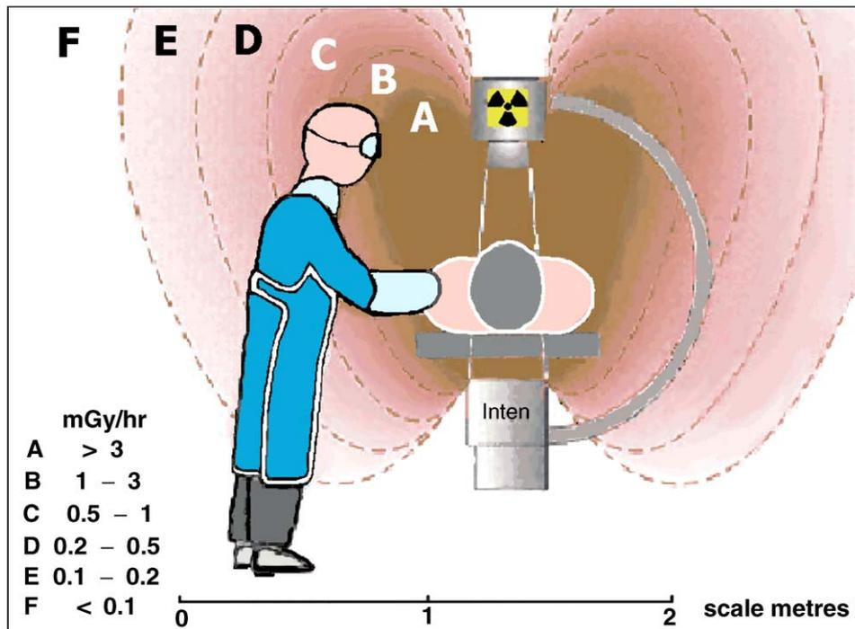
**Figure 3** With the X-ray generator above the table the maximal scatter is towards the surgeon's head and neck. Note that the scatter at the generator end of the C arm exceeds that at the receptor end. Compare with Fig. 4.
