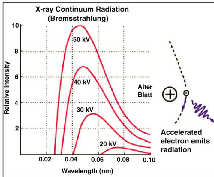
Figure 2 The bremsstrahlung continuous X-ray spectrum showing the effect of different voltages (kV).
